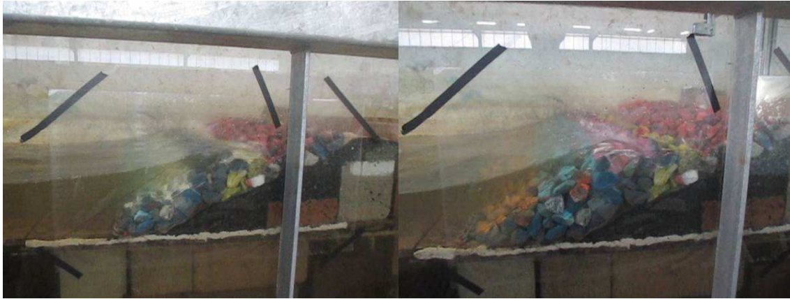
Figure 11 – Waves breaking on concept 3 during testing of base design (LHS) and adaptation strategy (RHS)
