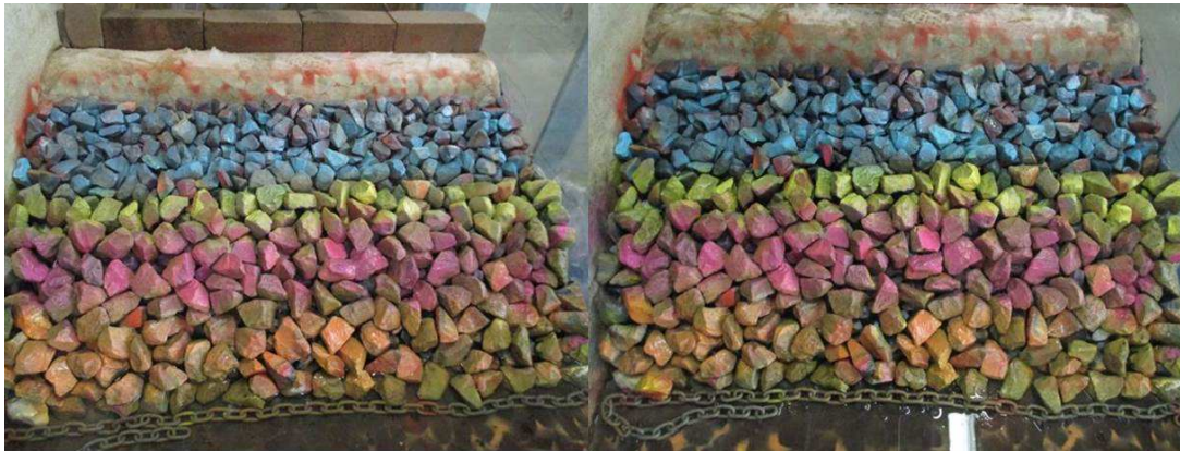
Figure 8 – Concept 2 before and after testing (0-1% damage)
