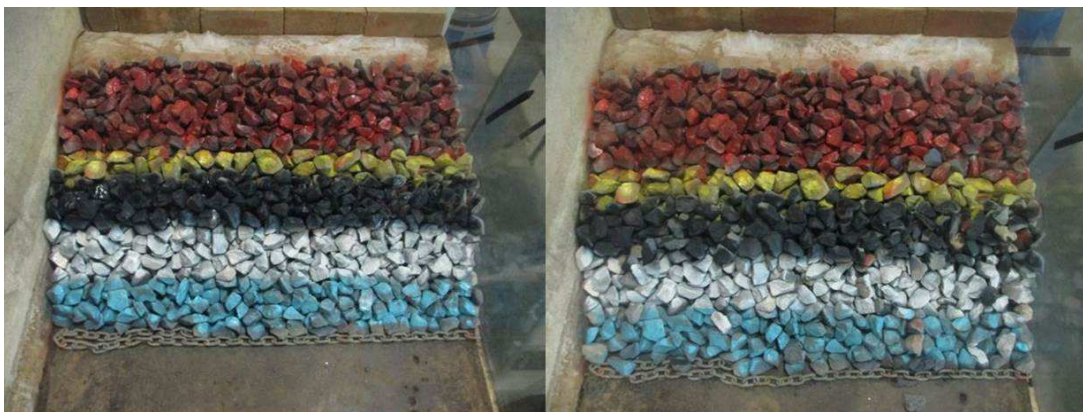
Figure 9 – Concept 3 before and after testing (1% damage)
