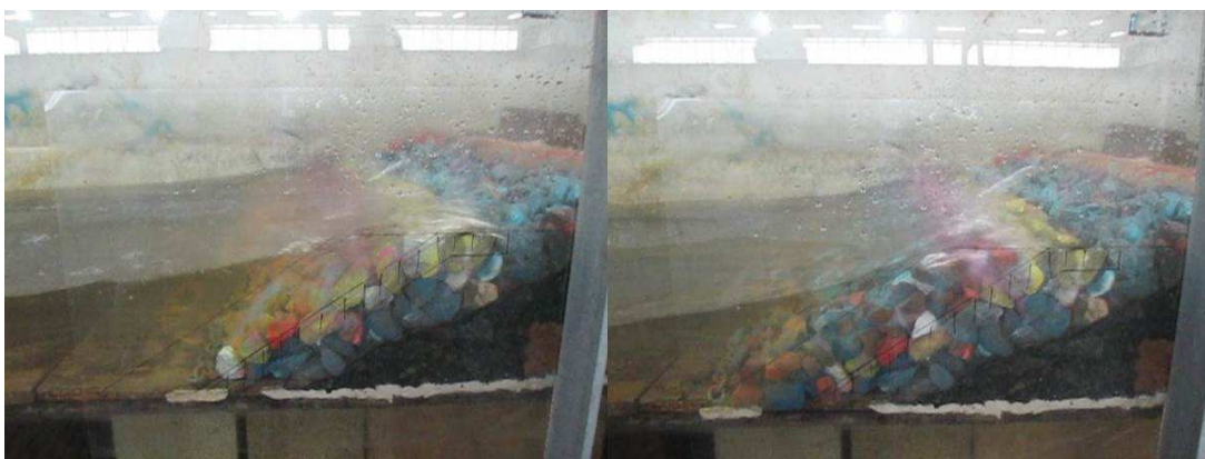
Figure 10 – Waves breaking on concept 2 during testing of base design (LHS) and adaptation strategy (RHS)
